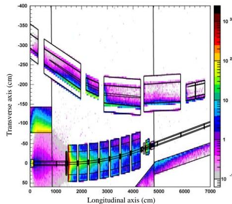
Figure 4: Top view of the simulated geometry after impact on TCDIV.87804. The values are in  $\text{mJ/cm}^3$ .
