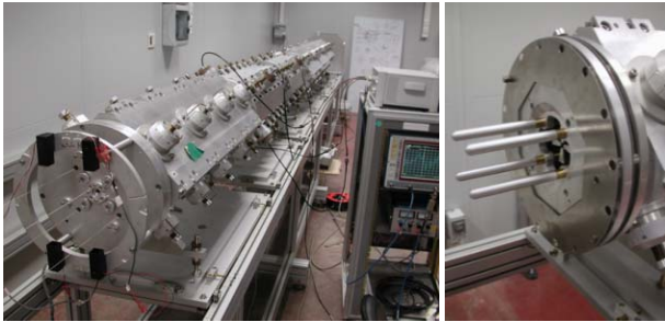
Figure 1 left: cold model with test bench Right: coupling cell with dipolar rods and 0.8mm shims on either side
