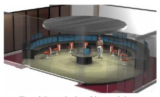
Figure 3, Isometric view of the console layout that can be used for access to personal email and video-conferencing. The entire console configuration encompasses 16 PCs and 40 LCD screens, and can easily be upgraded to double the number of PCs and/or add additional LCD screens.
