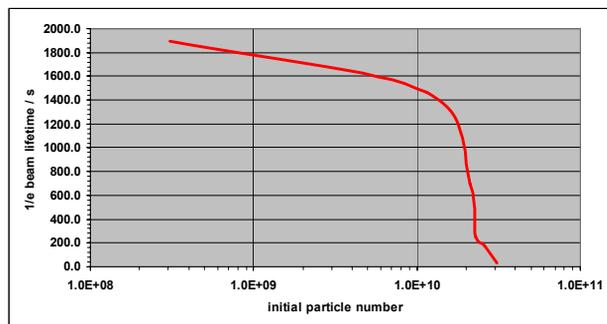
Figure 4: Beam lifetime of 45 MeV protons cooled with a 150 mA electron cooler beam current
