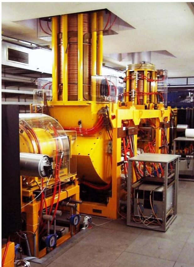
Figure 3: The COSY electron cooler
