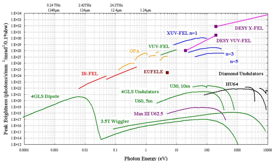
Figure 1. Peak brightness for 4GLS FELs, undulators, wiggler, OPA and dipoles compared with EUFELE, X-FEL, Diamond and Max III undulators.
