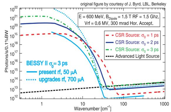
Figure 2: Comparison of scaled THz flux at BESSY by 3 ps bunches with simulated CIRCE parameters.
