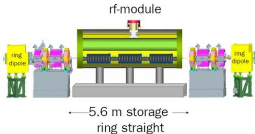
Figure 1: Scheme of a superconducting TESLA structure placed into one of the BESSY II straight sections.
