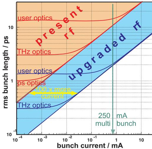
Figure 3: Bunch current relation for the present BESSY II ring (red) and extrapolated version with an 100x upgraded rf-gradient (blue).
