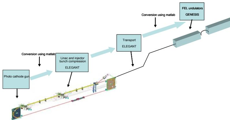
Figure 1: Overview of the FEL setup and start-to-end simulations.
