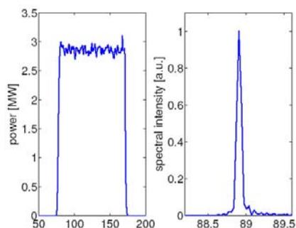
Figure 4: Temporal and spectral power distributions of FEL pulse at exit of radiator.
