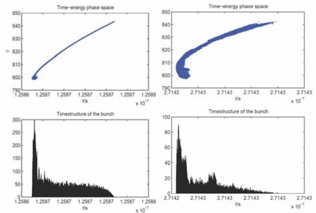
Figure 3: Left: Electron bunch after the recirculator, right: electron bunch before undulator section.
