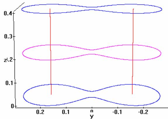
Figure 1: The CASSINI wires current undulator structure.
