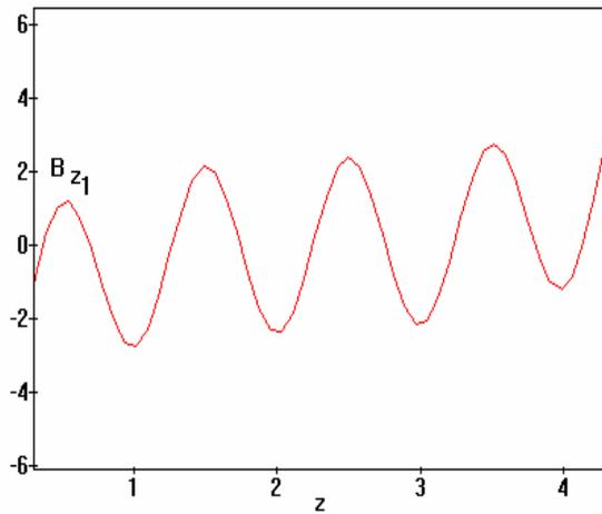
Figure 2: The undulator  $z$  magnetic field component vs.  $Z$  direction.
