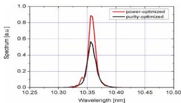
Figure 3: The dispersive sections in the HGHG cascade can be optimized to either yield high-power or high-purity output radiation.
