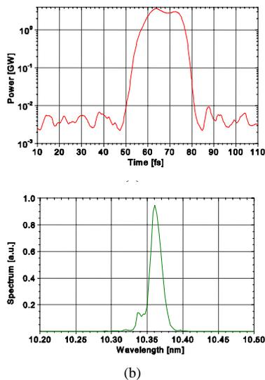
Figure 2: FEL pulse versus time and wavelength for the low-energy FEL.
