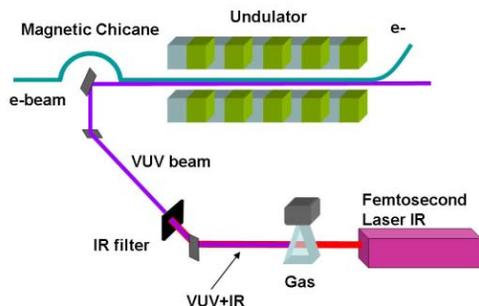
Figure 1: Experimental layout to seed harmonics generated in gas into FEL.
