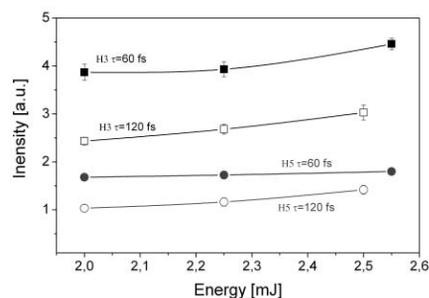
Figure 5: 3rd and 5th harmonics in argon as function of energy laser for two pulse width.
