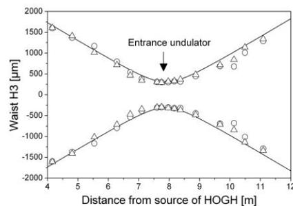
Figure 6: Longitudinal evolution of the beam waist of the 3rd harmonic in vertical ( $\Delta$ ) and horizontal ( $\circ$ ) direction. In solid line indicate the quasi-gaussian beam fit.
