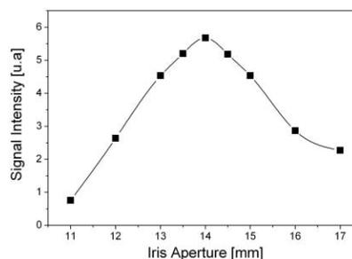
Figure 3: Harmonic signal as a function of aperture size.
