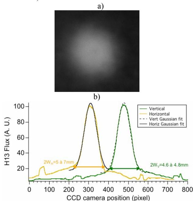
Figure 8: Transverse section (a) and profiles (b) of the 13<sup>th</sup> harmonics, 3 m after the cell but 8 m before the theoretical focusing point in the first undulator.
