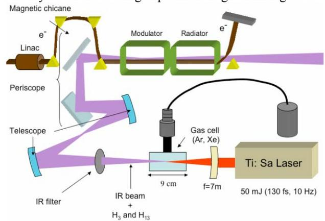
Figure 1: General layout of the seeding experiment with harmonics generated in a gas cell.
