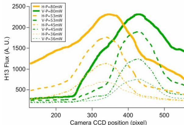
Figure 9: H<sub>13</sub> beam shape evolution as function of the IR power generated in Xenon gas with the 13 cm long cell. H and V are respectively for Horizontal and Vertical.
