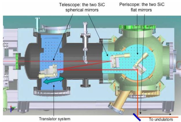
Figure 4: Refocusing system and periscope.
