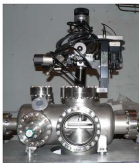
Figure 7: First chamber and harmonic generation cell.
