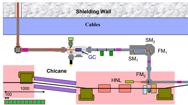
Figure 5: Location for the harmonic generation in gas experiment on the SCSS phase 1 machine. The drawing is at scale (unit: mm).
