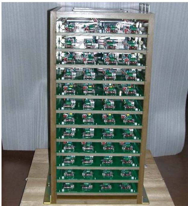
Figure 5: IGBT switching module constructed as an R&D for the bipolar fast extraction kicker system.
