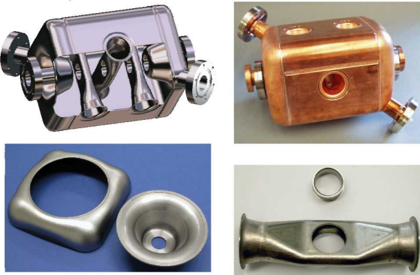
Figure 1: Triple-spoke cavity prototype – artistic view, copper model and Nb parts.
