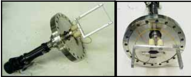
Figure 7: Picture of a horizontal scanning wire on the left and a vertical scanning wire on the right.
