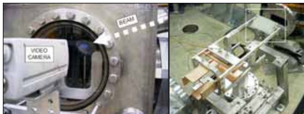
Figure 3: Pictures of the phosphor screen in the injection section (left) and in the extraction section (right).
