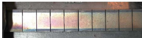
Figure 7: Mock-up after tests at 5 \text{ MWm}^{-2} , and a total of 2000 cycles.
