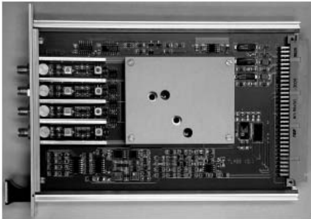
Figure 3: The RF signal processing front-end unit.
