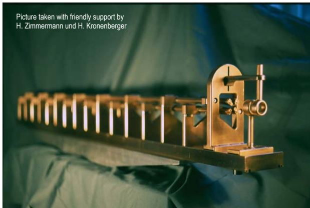
Figure 1: The RFQ-Drifttube-Combination right before its installation into the tank.
