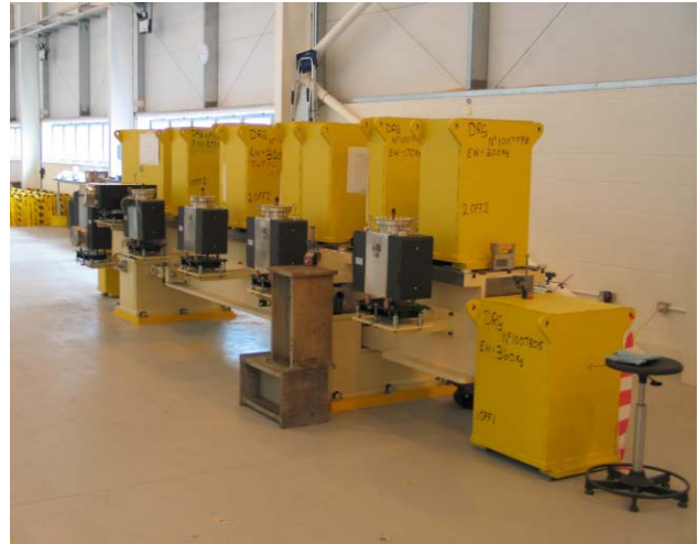
Figure 2: Prototype girder undergoing tests in the new Diamond assembly building.
