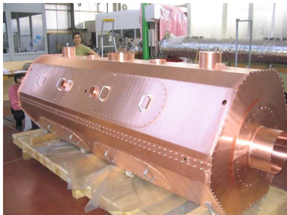
Figure 2: Copper thermal shield with 8 dismountable access doors.
