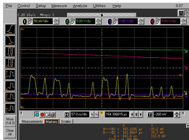
Figure 3: “C” ( -.-. ) “L” ( -.-. ) “S” ( ... ) storage ring injection profile.
