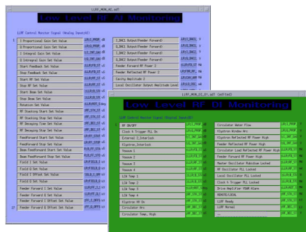
Figure 7: EPICS Extensions of RF control system
