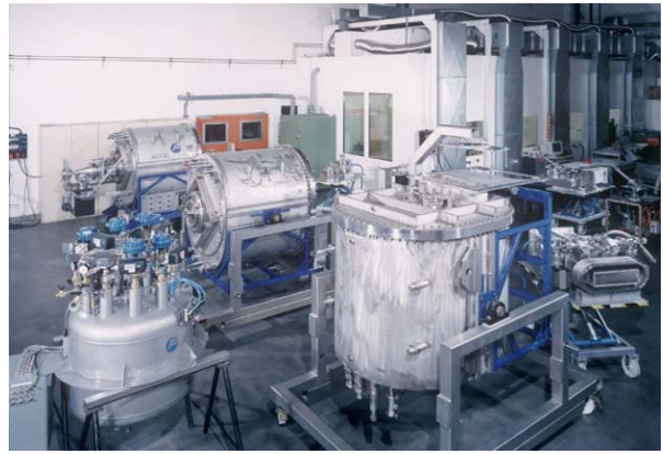
Figure 3: Assembly area of the SRF modules at ACCEL. In the upper right part the clean room class 100 can be seen where the modules need to be assembled in whenever the cavity vacuum is touched.
