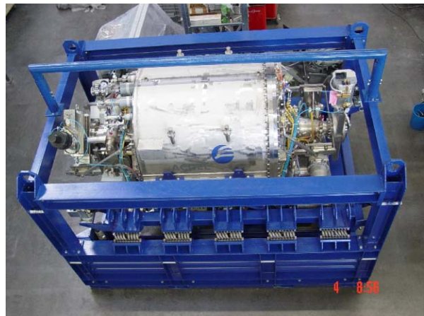
Figure 4: Completed SRF module for Cornell University installed into shipping frame.
