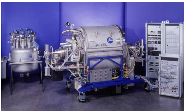
Figure 2: Superconducting accelerator module for the Taiwan Light Source with valve box (left) and SRF electronics (right) prior shipment to NSRRC.
