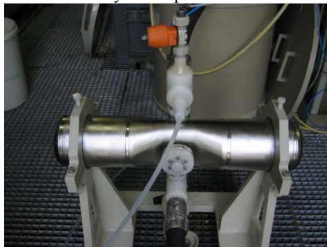
Figure 9: First HWR 176 MHz cavity during chemical treatment at ACCEL.
