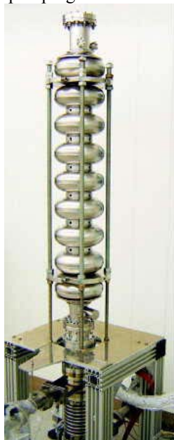
Figure 6: High pressure rinsing of a nine cell 1300 MHz TESLA cavity at ACCEL.
