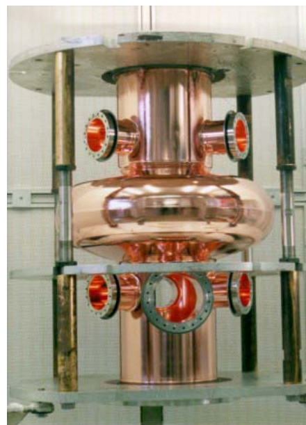
Figure 1: Single cell 400 MHz LHC cavity before sputtering with niobium.
