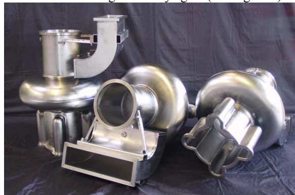
Figure 4: Three 500 MHz cavities of the Cornell design after production and prior preparation.
