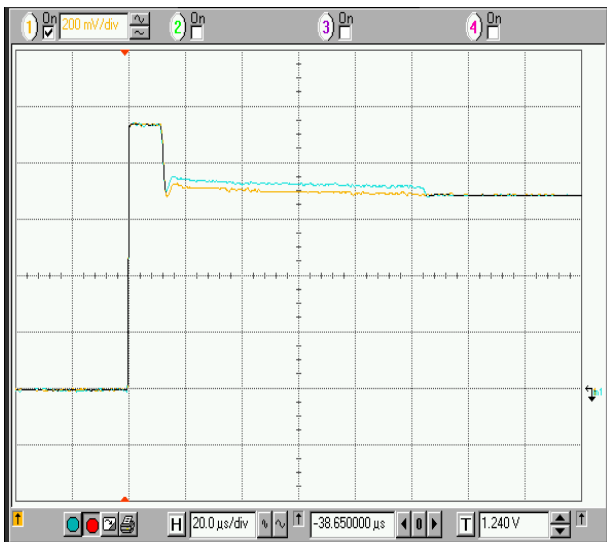
Figure 7: Step response of output signal with (bottom) and without (top) integrator anti-windup.
