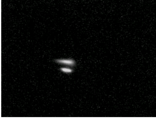
Figure 2: Synchrotron light image in Arc-1, showing the presence of the accelerated and energy recovered beam.
