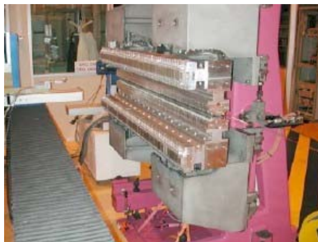
Figure 2: ESRF revolver prototype before installation in the ID18 straight section, the support is equipped with a U32 and a U20.
