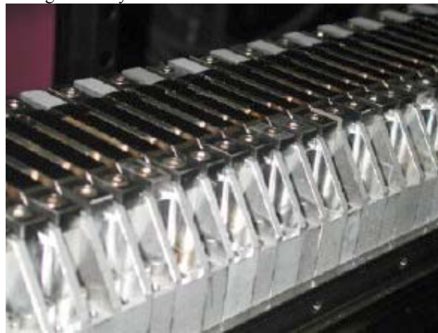
Figure 4: Hybrid magnetic structure of the U22 in-vacuum undulator.
