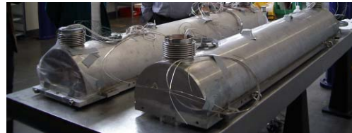
Fig. 2 Vacuum vessel (insulation vacuum) for each of the coils. The correction coils are also inside the vacuum vessel
