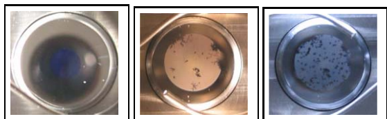
Figure 4: Surface of two cathodes. Left, cathode 42.2 after 80 days of operation at TTF, cathode 60.1 after 2 month (middle) and 4 month of operation (right) in the present gun at PITZ.
