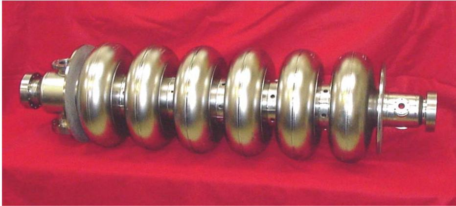
6 cells  $\beta=0.81$  cavity 6SNS81-1 stiffening ring at 80mm
