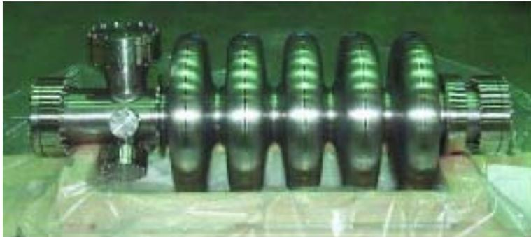
Fig. 1 600MHz 5-cell cavity ( $\beta=0.604$ )
