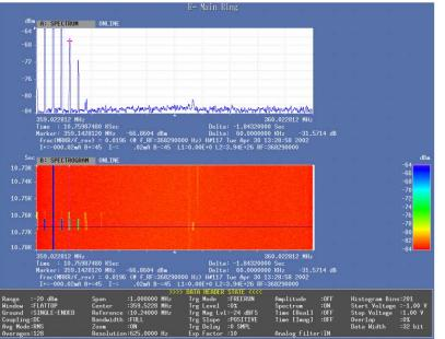
• Besides, there is another peculiar aspect: considering the multibunch case (Vrf=120kV), the quadrupole frequency (58.75KHz) has a frequency shift by -1.25 kHz relatively to the second harmonic of the synchrotron frequency (60kHz)
