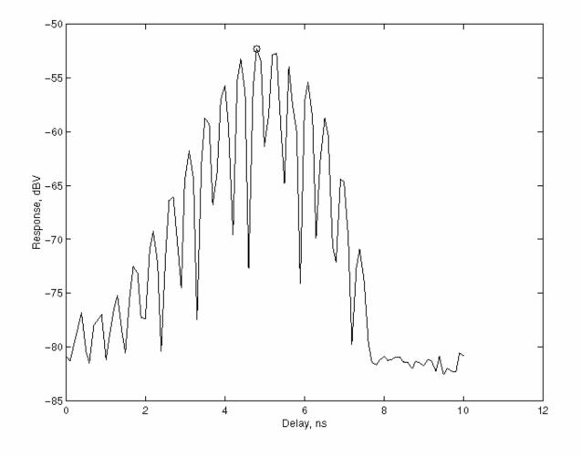
This is the longitudinal backend response versus delay; The bunch passage should be synchronized with the center of the highest lobe to exploit the most of the power.
