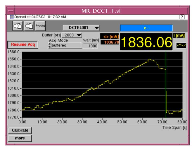
More then 1.1 A injected and stored in collision in each ring (47 bunches, November 2001)
