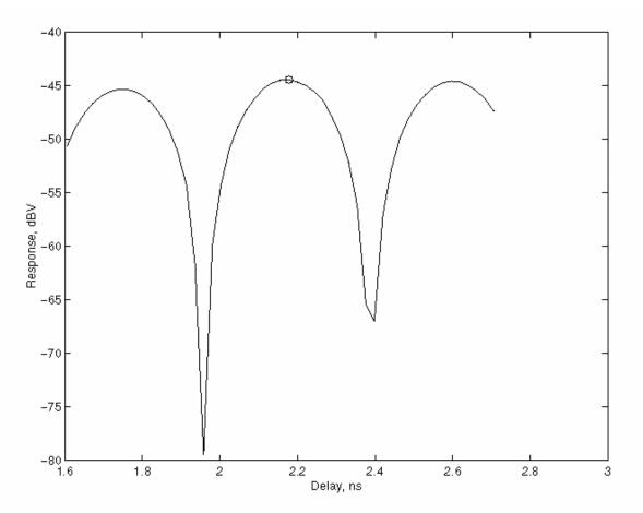
Measuring the q-pole threshold versus LFB backend delay, we discover that increasing delay (kicking bunch tail) produces higher or no thresholds and decreasing delay (kicking bunch head) lowers q-pole threshold.
