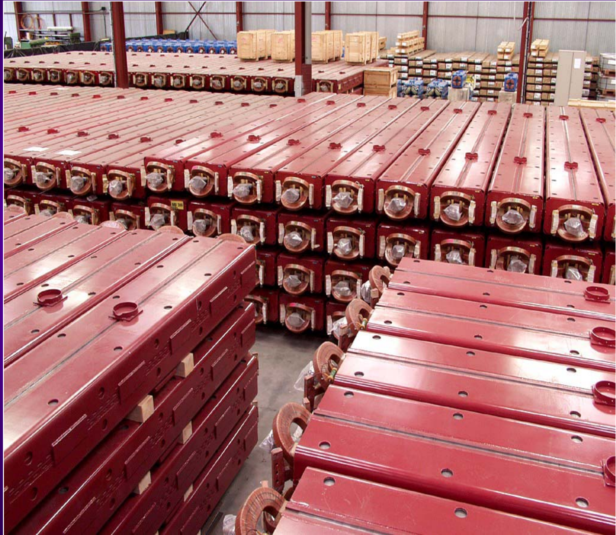
Dipole magnets waiting for installation
