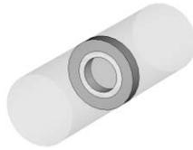
Figure 1: Cylindrical resonator including a dielectric ring covered with a gyrotropic material
