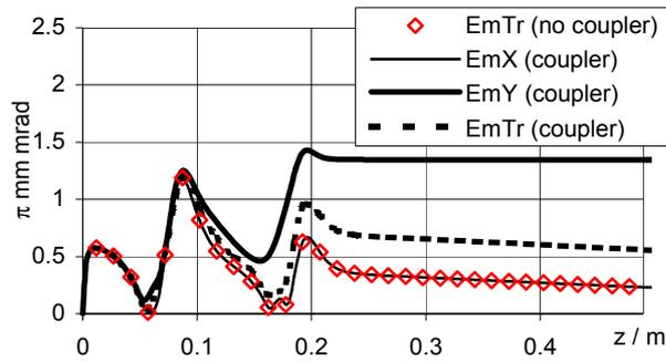
Figure 5: RF induced beam emittance.
