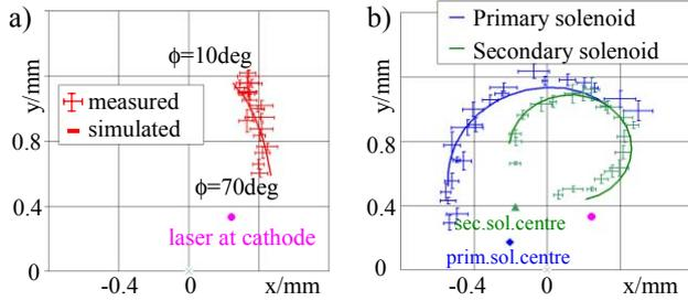
Figure 3: Beam position as a function of: a) rf phase; b) primary and secondary solenoid current.
