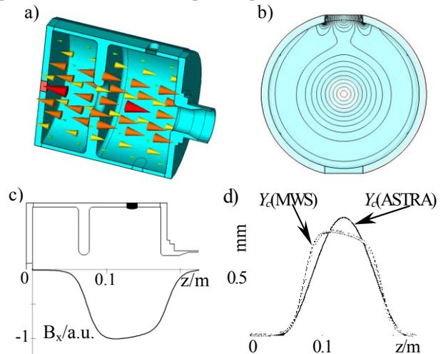
Figure 2: a) Electric field of the  $E_{01}-\pi$  mode; b)  $E_{01}-\pi$  mode magnetic field isolines in the coupler cross section; c) Horizontal component of magnetic field on the cavity axis; d)  $E_{01}-\pi$  mode offset.
