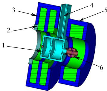
Figure 1: TTF rf gun layout: 1–rf cavity, 2–trim coil, 3–primary solenoid, 4–power coupler, 5–secondary solenoid, 6–beam position monitor BPM1 .
