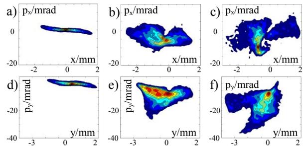
Figure 8: Transverse phase spaces  $(x,p_x)$  and  $(y,p_y)$  at longitudinal position  $z=1.5m$ : a),d) -case 3 (no rf kick) from the Table; b),e) -case 3 (with rf kick); c),f) -case 4.
