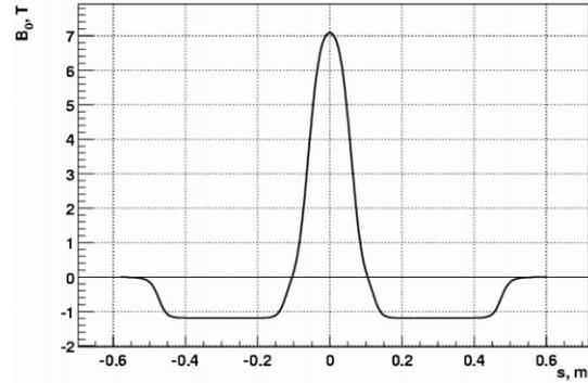
Fig.4.1 Vertical magnetic field along the wiggler axis.
