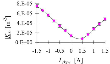
Figure 2: Modulus of the normalised skew gradient, as deduced from tune separation measurements, vs. skew quadrupole current for the PS at injection energy.
