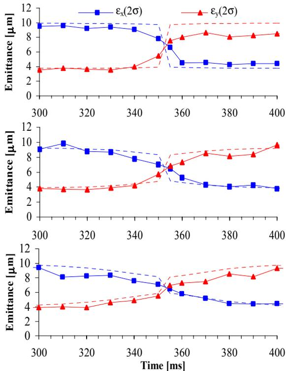
Figure 4: Transverse physical emittances vs. time for  $I_{skew} \approx 0.1$  A (upper),  $I_{skew} \approx -0.5$  A (centre), and  $I_{skew} \approx -1.5$  A (lower). The dashed lines denote the theoretical values and the solid lines the measured ones.
