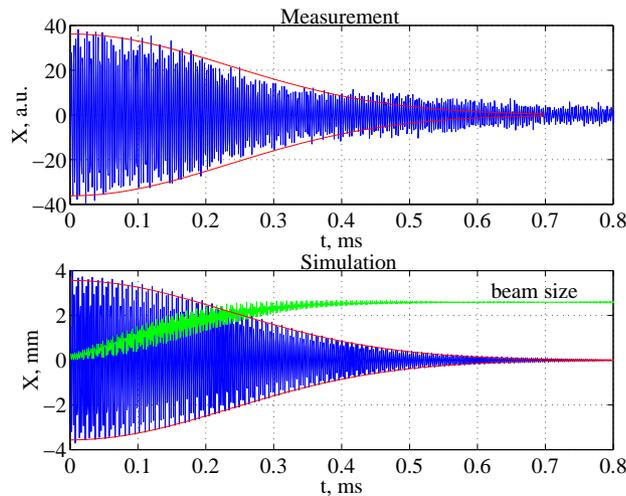
Figure 4. Gaussian damping of the coherent oscillation
