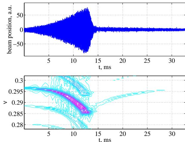
Figure 1. Horizontal instability at S1 = 50 A
