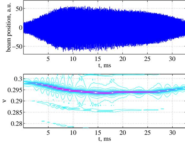
Figure 2. Horizontal instability at S1 = 40 A
