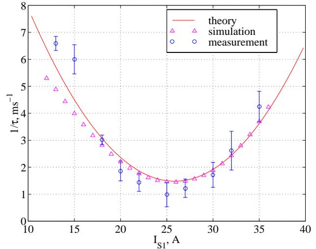
Figure 5. Damping rate vs harmonic sextupole current
