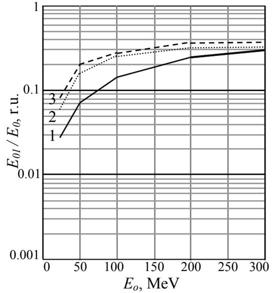
Figure 4: Bremsstrahlung output dependences on electron energy. Number of targets - 10. Registration cone  $\theta=5^\circ$ .
