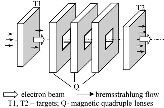
Figure 1: The scheme of magnetic system for a bremsstrahlung source with thin targets.
