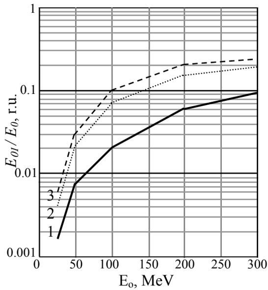
Figure 2: Bremsstrahlung output dependences on electron energy. Number of targets - 10. Registration cone  $\theta=1^\circ$ .
