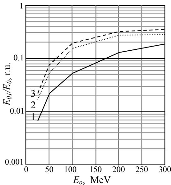
Figure 3: Bremsstrahlung output dependences on electron energy. Number of targets - 10. Registration cone  $\theta=2^\circ$ .
