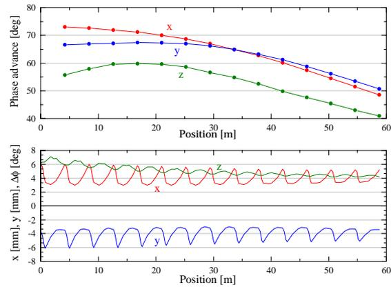
Figure 2: Phase advances and beam envelopes for a 30 mA beam in the first section of the TRASCO linac. The beam is matched with the adiabatic procedure.
