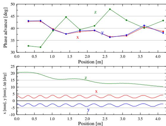
Figure 3: Phase advances and beam envelopes for a 50 mA beam in a DTL tank (from 2.5 to 7.5 MeV). The beam is matched with periodic conditions.
