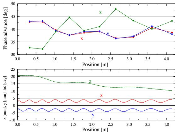
Figure 3: Phase advances and beam envelopes for a 50 mA beam in a DTL tank (from 2.5 to 7.5 MeV). The beam is matched with periodic conditions.
