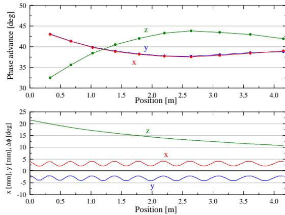
Figure 4: Phase advances and beam envelopes for a 50 mA beam in a DTL tank (from 2.5 to 7.5 MeV). The beam is matched with the adiabatic procedure
