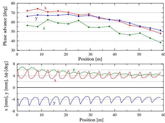
Figure 1: Phase advances and beam envelopes for a 30 mA beam in the first section of the TRASCO linac. The beam is matched with periodic conditions.
