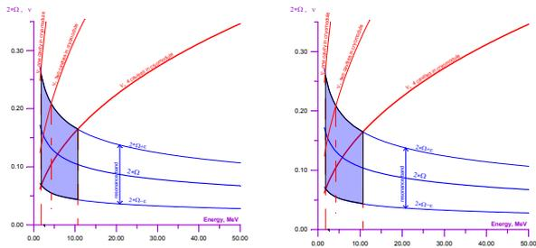
Figure 5: The parametric resonance for H and D beams due to the proposed drift space in the HWR linac.
