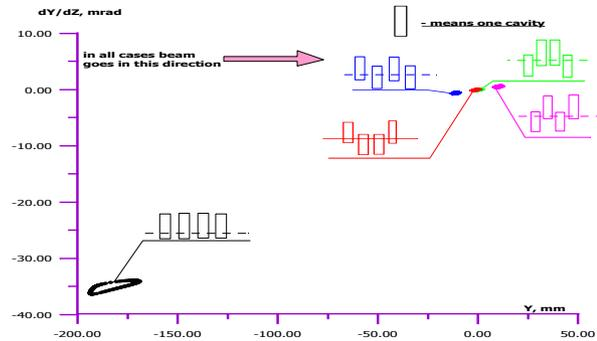
Figure 1: X,  $dx/dz$  position of beam for different schemes of compensation.
