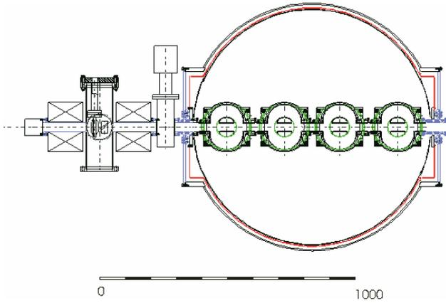
Figure 2: One unit cell of linear accelerator
