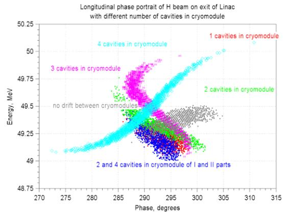
Figure 6: Phase portraits of H beam at the exit of the HWR linac, assuming different arrangement options.
