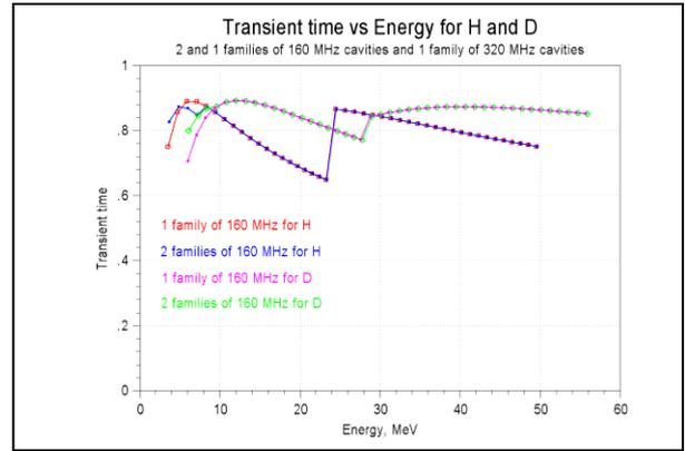
Figure 4: Transient time for H and D beams (44 cavities totally).
