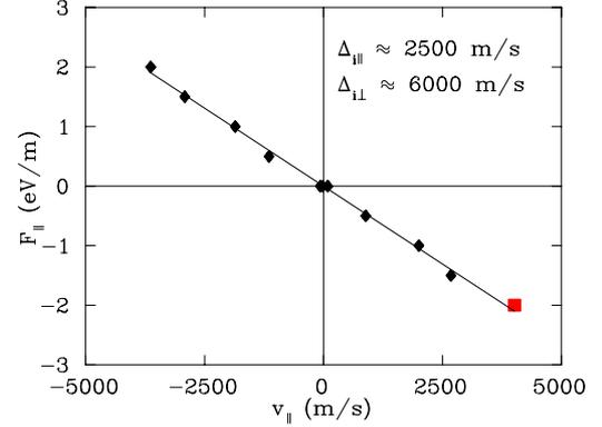
Figure 3: Longitudinal cooling force as function of the longitudinal relative velocity ( $^{12}\text{C}^{6+}$ , 73.3 MeV,  $I_{ion} = 20 \mu\text{A}$ ,  $n_e = 8 \cdot 10^6 \text{ cm}^{-3}$ ).  $\Delta_{i\parallel}$  is the longitudinal and  $\Delta_{i\perp}$  the transverse velocity spread of the ion beam.
