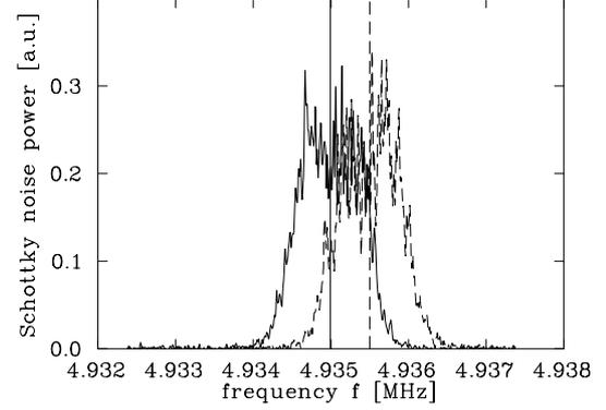
Figure 2: Longitudinal cooling force measurement with the IndAcc. Full curve is the spectrum of the cooled beam. Applying  $U_{ind} = 0.4 \text{ V}$  results in a spectrum shown by the dashed curve. The first momenta are drawn as straight lines.
