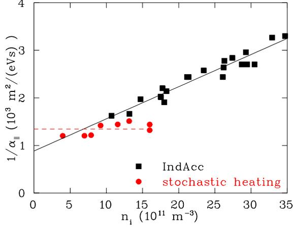
Figure 4: Inverse friction coefficient  $1/\alpha_{\parallel}$  as function of the average ion density for  $^{12}\text{C}^{6+}$  ions ( $E = 73.3$  MeV,  $n_e = 8 \cdot 10^6 \text{ cm}^{-3}$ ). Measurements with the induction accelerator (squares) and with stochastic heating (circles) are shown. To the IndAcc data a linear function is fitted (full line), while the data obtained with stochastic heating is well represented by a constant function (dashed line).
