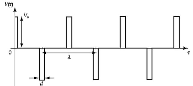
Figure 2: Example pattern of the electrode voltage  $V(\tau)$ .
