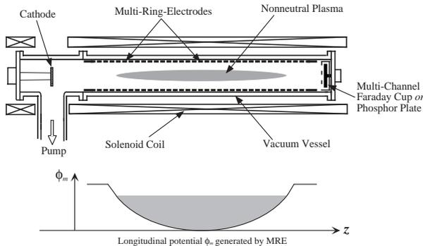
Figure 3: A multi-ring-electrode trap
