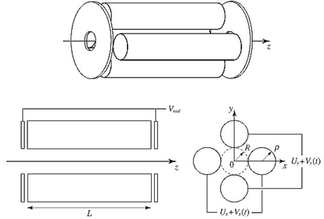
Figure 1: Schematic view of a typical Paul trap.
