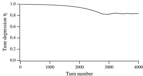
Figure 2: Time evolution of tune depression during a cooling process.
