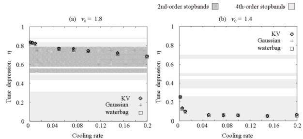
Figure 3: The lowest tune depression vs. cooling rate  $\zeta_{\perp}$ . The ordinate indicates the minimum tune depression at which the tune locking occurred. We have considered a 1 MeV  $^{24}\text{Mg}^+$  beam cooled in the TARN II lattice.
