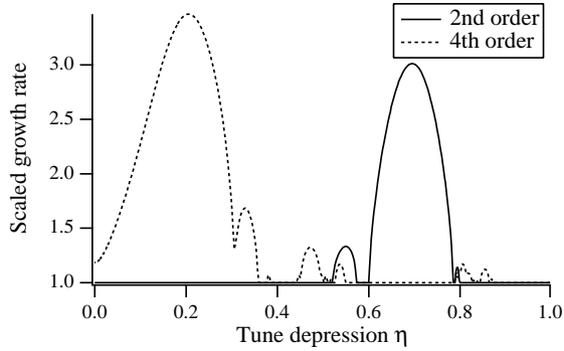
Figure 1: Resonance stopbands calculated from the 2D Vlasov-Poisson equations. The solid line expresses the growth rate of instability due to second-order resonances while the broken line that due to fourth-order resonances.
