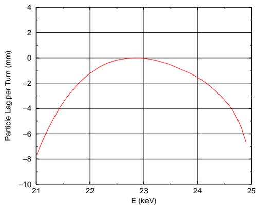
Figure 4: Particle lag per turn behind a reference particle vs. energy. The kinetic energy of the reference particle is 22.8 keV.
