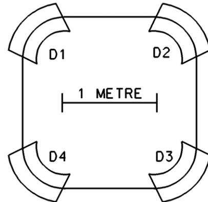
Figure 1: Bare SIR lattice, shown without steering, inflector and deflector plates.
