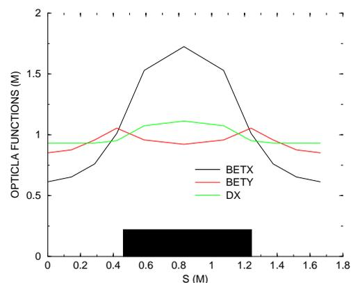
Figure 2: The optical functions for a single period of SIR vs. distance. The solid rectangle schematically shows one of the  $90^\circ$  dipole magnets.
