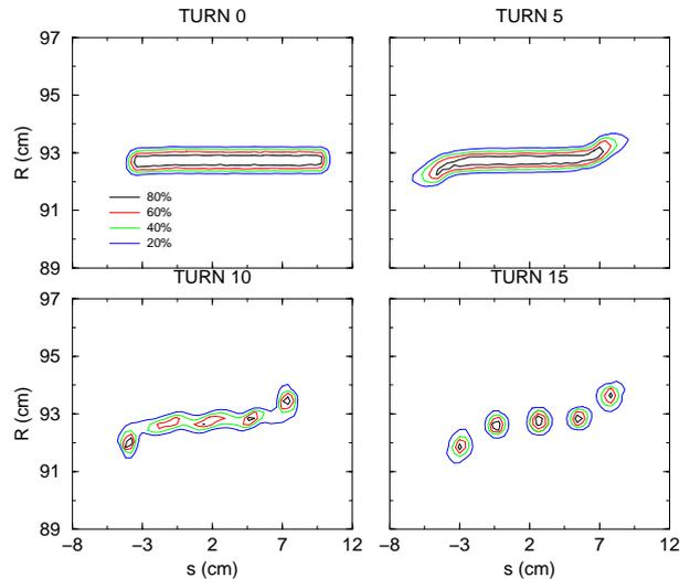
Figure 7: Median-plane charge density contour plot of the 22.8 keV, 16  $\mu$ A deuteron bunch in SIR after 0 (initial distribution), 5, 10, and 15 turns.
