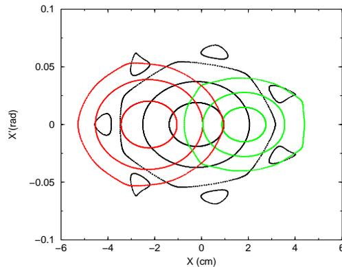
Figure 5: X-X' phase space plot at the mid-point of a drift between magnets. Different colors correspond to different particle energies: red to 21.8 keV, black to 22.8 keV, and green to 23.8 keV.
