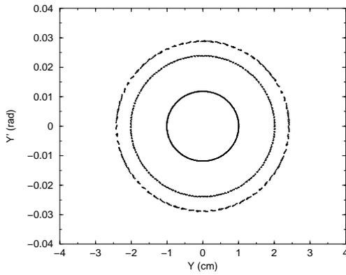
Figure 6: Y-Y' phase space plot at the mid-point of a drift between magnets.
