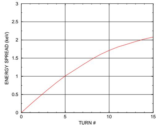
Figure 8: Energy spread with the bunch as a function of the turn number.
