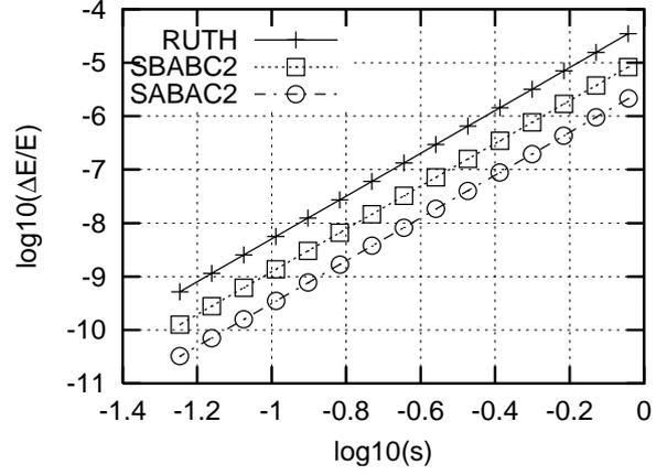
Figure 1: Relative energy error versus integration step size in logarithmic scale. The integrators  $SABA_2$  and  $SBAB_2$  with correctors are more precise than the Forest and Ruth  $S_4$  integrator by respectively one order and half a order of magnitude at the same cost.
