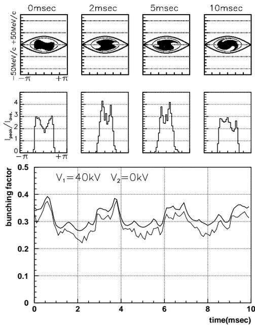
Figure 1: Simulation result with  $V_1=40\text{kV}$ . Phase-space distribution(top), bunch profile(middle) and bunching factor(bottom) with(thick) and without(thin) smoothing as functions of time.
