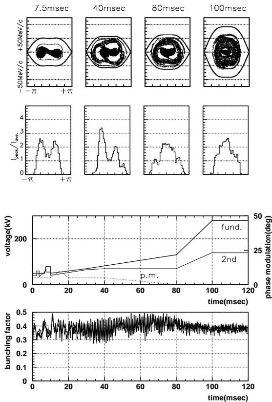
Figure 3: Simulation result for emittance blow-up. Mismatch excitation and phase modulation are used here. Phase-space distribution(top), program of the rf-voltages and phase modulation(middle), and bunching factor(bottom) are shown as functions of time.
