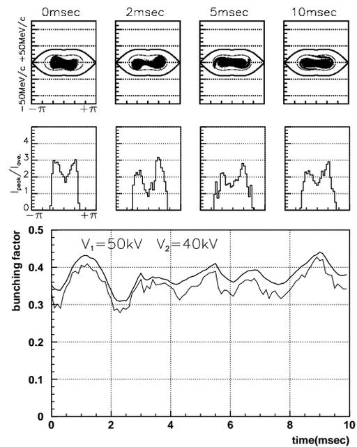
Figure 2: Simulation result with  $V_1=50\text{kV}$  and  $V_2=40\text{kV}$ . Phase-space distribution(top), bunch profile(middle) and bunching factor(bottom) are shown as functions of time.
