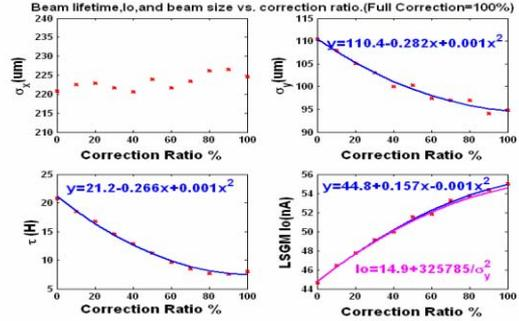
Figure 9: Horizontal and vertical beam sizes, synchrotron light intensity from a pinhole measurement, beam lifetime (from top left to right left in clockwise) as a function of the correction ratio, assuming full correction is 100%.
