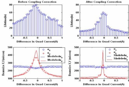
Figure 7: Measured and modeled beam size as well as lifetime as a function of the quadrupole Q2 strength.
