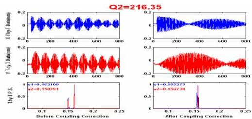
Figure 5: Measured turn-by-turn data after a horizontal kick and the corresponding tune spectra near the coupling resonance before and after corrections.
