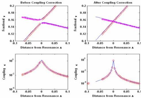
Figure 8: Extracted coupling ratio as a function tune difference from the resonance point.
