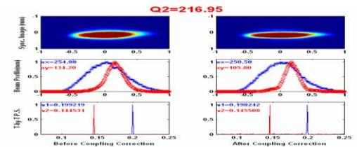
Figure 6: Measured beam images and corresponding tune spectra in the routine operations before and after
