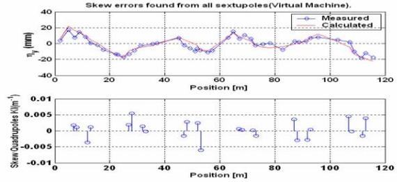
Figure 3: Assuming all errors are from sextupoles, a virtual machine is obtained using SVD method. Measured and model vertical dispersion is also shown.
