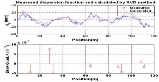
Figure 2: Correction strength of skew quadrupoles and a comparison between experiment and model in vertical dispersion.
