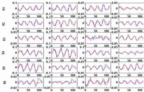
Figure 1: Measured vertical orbit response with respect to the corresponding horizontal kick as well as calculated
