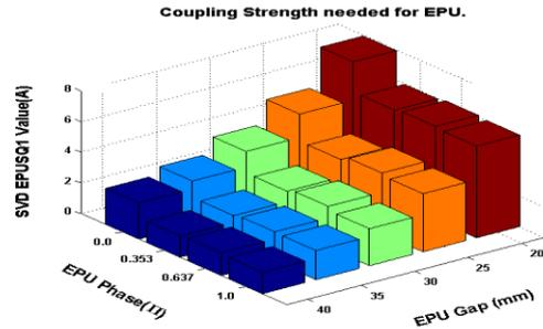
Figure 10: Additional required skew quadrupolar strength to accomplish the correction as the EPU gap and phase are varied.
