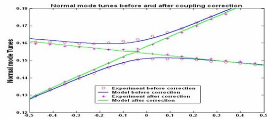
Figure 4: Experimental and model normal mode tunes, before and after correction.
