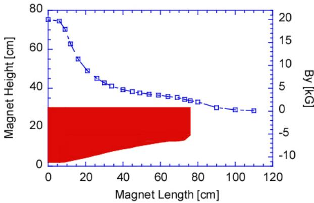
Fig. 2 Profile and field distribution of variational bend in Table 1 with 2.0 Tesla max B, without transverse gradient
