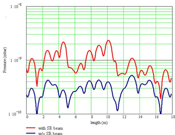
Figure 5: Pressure profile along the arc.
