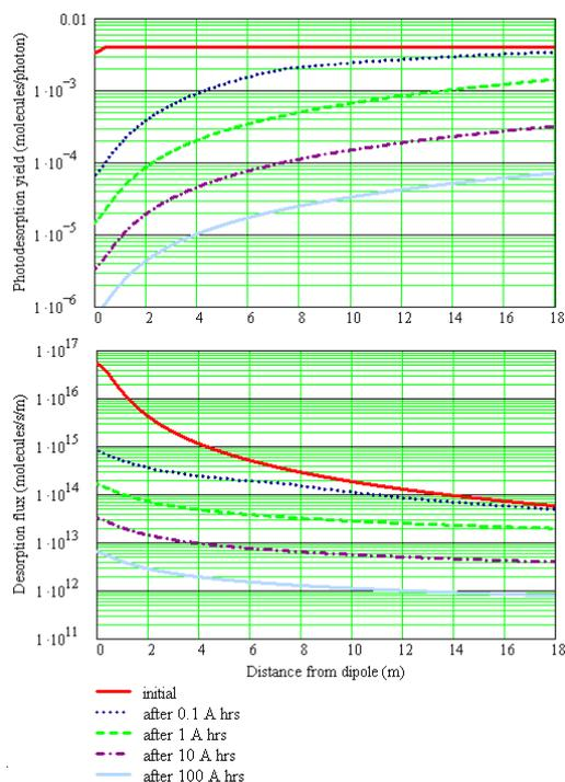
Figure 4: Photo-desorption yield and desorption flux for a straight irradiated by SR from dipole as a function of distance from the dipole and of beam dose.
