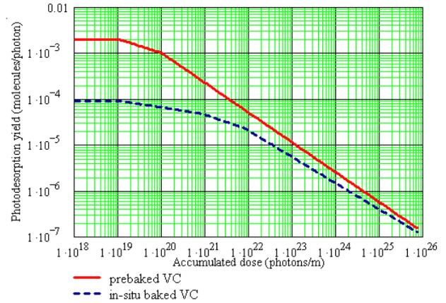
Figure 3: PSD yield for CO for prebaked and *in-situ* baked vacuum chambers. (Yields for doses higher than  $10^{23}$  photons/m are extrapolations.)
