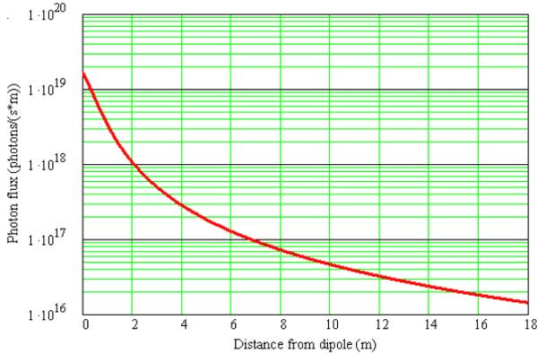
Figure 2: Photon flux incident on the vacuum chamber walls as a function of distance downstream from a dipole.
