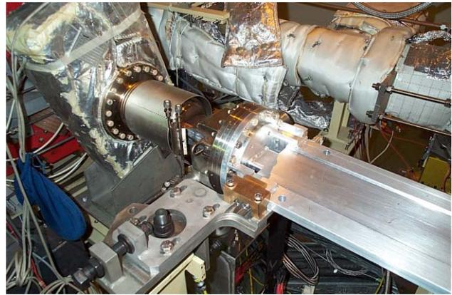
Figure 2d: Close-range view of the "10 mm", extruded-aluminium CV5073 installed on ID6 (right).
