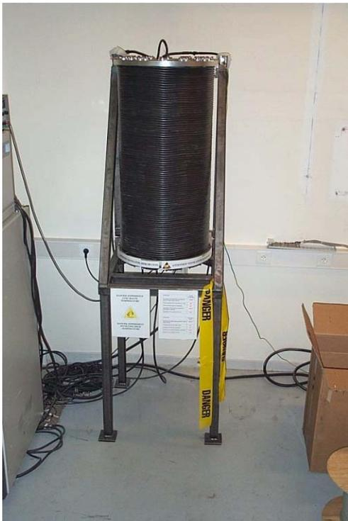
Figure 3b: Air-cooled solenoid for magnetron sputtering
