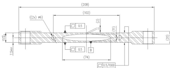
Figure 2b: 15 mm, extruded-aluminium vacuum chamber.
