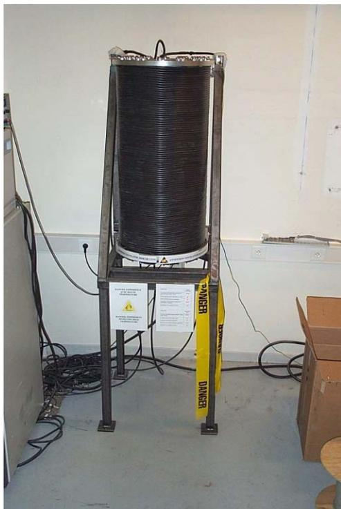
Figure 3b: Air-cooled solenoid for magnetron sputtering
