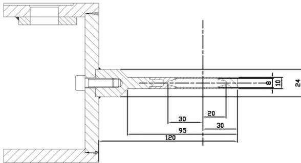
Figure 2c: 10 mm, stainless steel vacuum chamber. Two versions exist, with 50 and 57 mm horizontal apertures, respectively.
