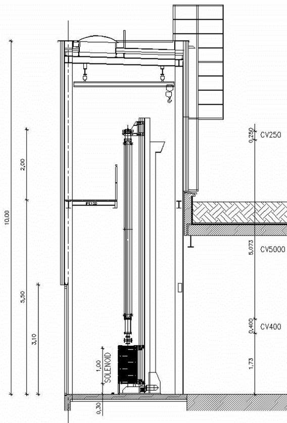
Figure 3a: Set-up for magnetron sputtering of a 5 metre long vacuum chamber.
