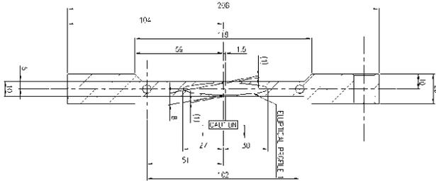
Figure 2a: 10 mm, extruded-aluminium vacuum chamber.
