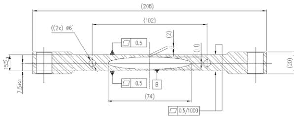
Figure 2b: 15 mm, extruded-aluminium vacuum chamber.
