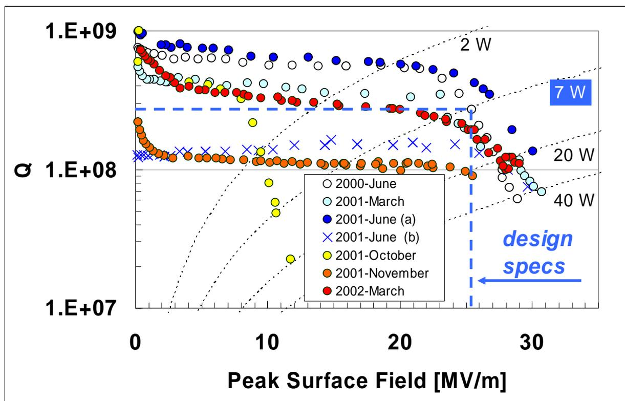
Figure 2: Evolution in the performance of SRFQ2, during the tests performed in the last two years.
