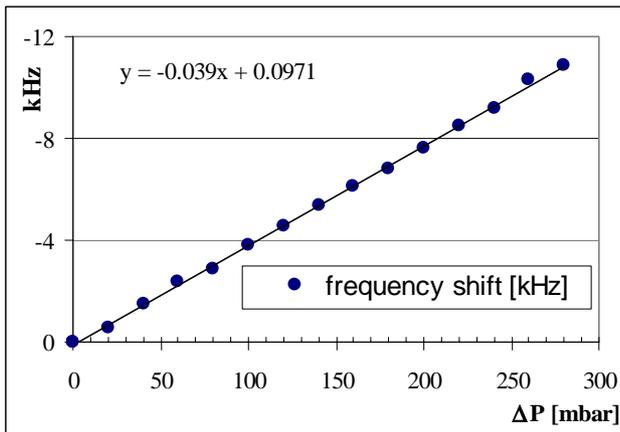
Figure 3: Frequency shift induced by He bath pressurization.
