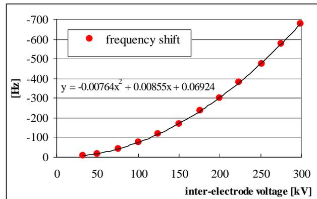
Figure 4: SRFQ2 resonance frequency shift is shown as a function of the inter-electrode voltage.
