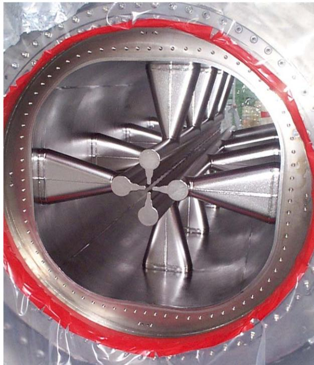
Figure 1: The newly built 1.34 m long SRFQ1 resonator during HPWR, preceding the sc tests.
